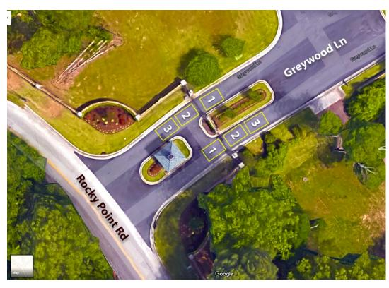
The **first** sensor area is the **APPROACH** area (**1**) which is the area right in front of the gate.
